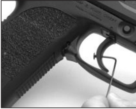
Fig. 28 Trigger stop adjustment with 1.5 mm Allen (hex) wrench
