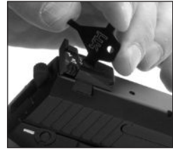
Fig. 30 Adjusting elevation screw
