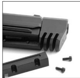
Fig. 36 Counterweight base and screws
