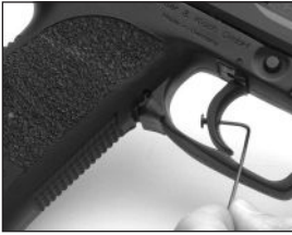
Fig. 28 Trigger stop adjustment with 1.5 mm Allen (hex) wrench
