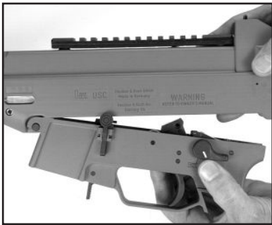
Fig. 23 Detaching lower receiver
