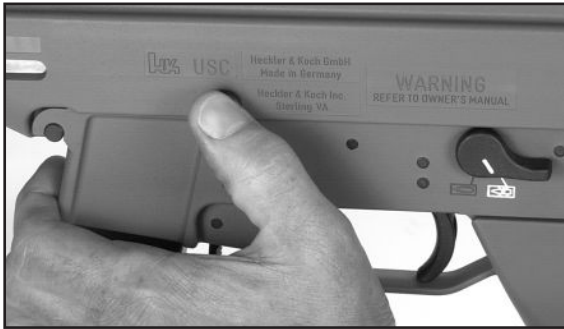
Fig. 21 Depress bolt catch to release the bolt
