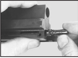
Fig. 28 Insert firing pin spring and firing pin assembly
