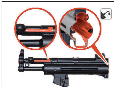
Fig. 50 – Lubrication points of functional elements
