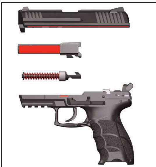
Figure 42 — Lubrications Points (in red)
