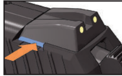
Figure 16 — Adjusting rear sight by lateral shifting
