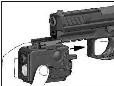
Figure 48 — Installing accessory onto the rails
