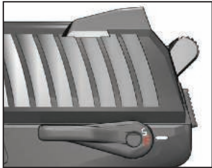
Figure 9 Safety lever in FIRE position
