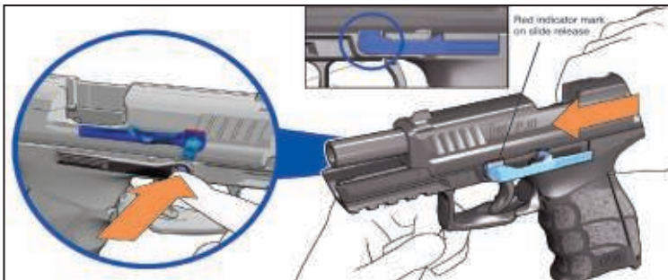
Figure 23 — Removing slide from frame by pushing it forward
