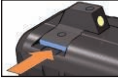
Figure 15— Adjusting front sight by lateral shifting
