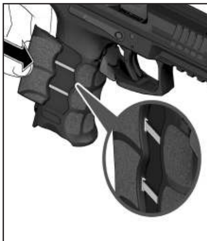
Figure 12 Push the grip panels forward onto the guide rails on the frame
