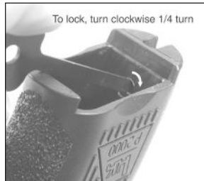
Figure 27 Turning the key clockwise 1/4 turn locks the action, turning it counter-clockwise unlocks the action.
