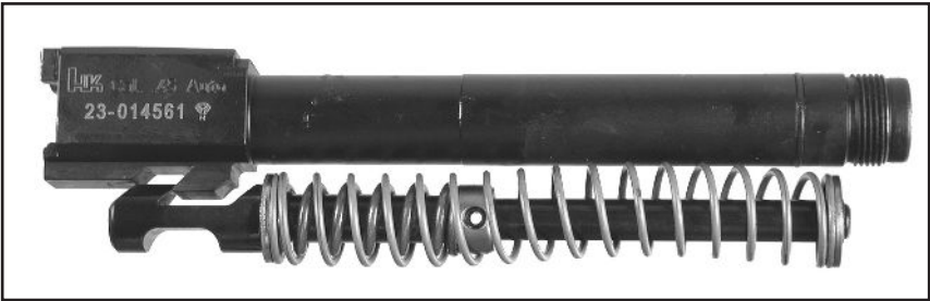
Figure 12 - Proper Position for the Captured Recoil/Buffer Spring Assembly on the Barrel Locking Block
