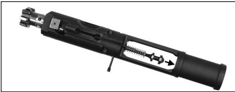
Fig. 42 – Removing the Firing Pin and Firing Pin Spring from the Bolt Assembly
