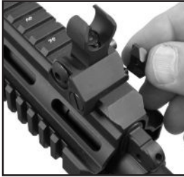
Fig. 6 – Installing front TROY sight Fig. 7 – Tightening front TROY sight
