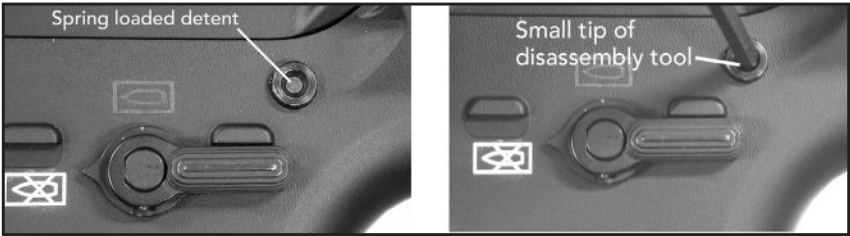
Fig. 68 – Detail of the rear Takedown Pin showing spring loaded detent.
