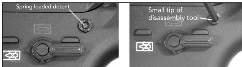
Fig. 66– Detail of the rear Takedown Pin showing spring loaded detent.
