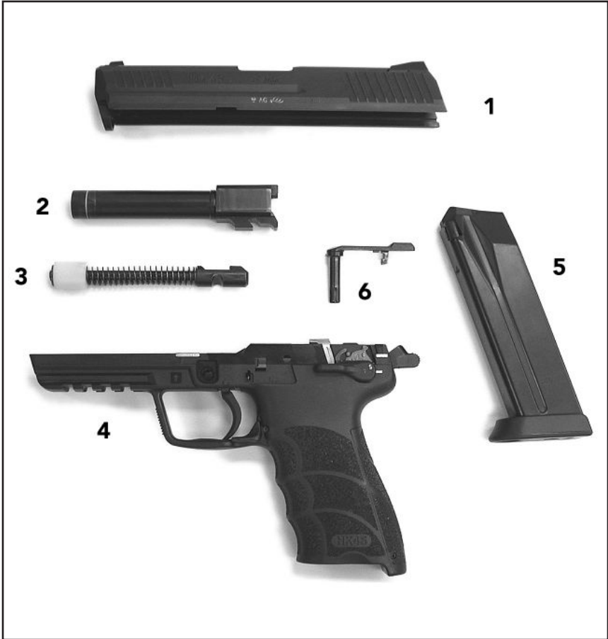
Figure 22 HK45 fieldstripped into Major Assembly Groups
