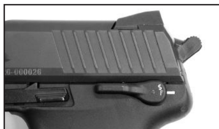
Figure 5 Control lever in “fire” position
