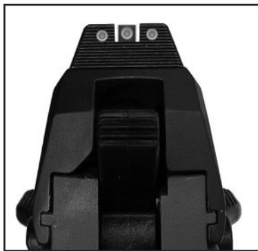
Figure 7 Rear and front sight aligned
