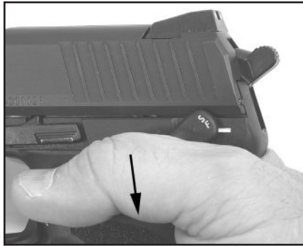
Figure 6 Control lever in “decocking” position
