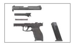
The VP pistols can be easily field stripped and disassembled without the need to pull the trigger prior to removing the slide. A low maintenance design, the VP has a service life of many tens of thousands of rounds.
