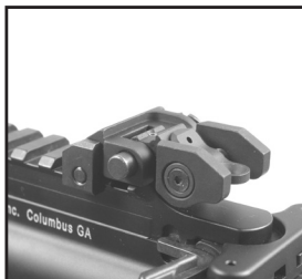
Fig. 12 – Rear sight folded (lowered)
