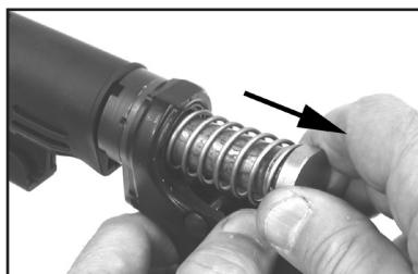
Fig. 95 – Removing non-HK Buffer and Action (Recoil) Spring
