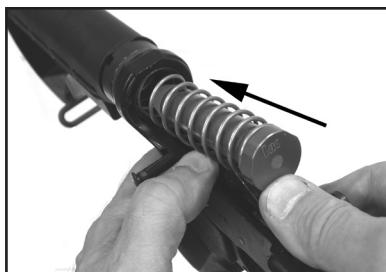
Fig. 96 – Installing HK Buffer and Action (Recoil) Spring
