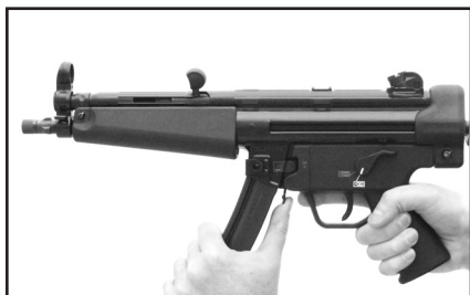
Fig. 27 – Depress the SP5 magazine release lever or button.
