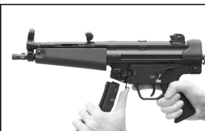
Fig. 28 – Remove the magazine from the magazine well.
