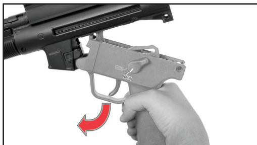
Fig. 34 – Remove trigger group
