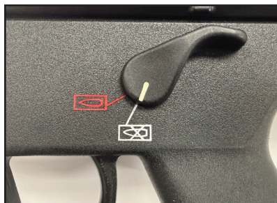
Fig. 4 – Selector lever on SAFE
