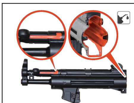
Fig. 49 – Lubrication points of functional elements
