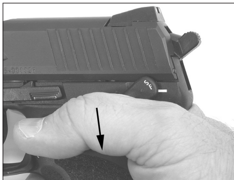
Figure 6 — Safety lever in "decocking" position
