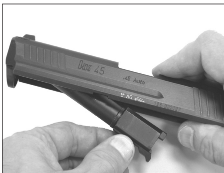
Figure 20 — Remove locking block
