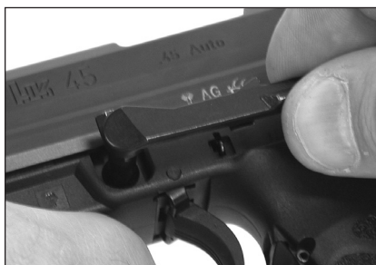
Figure 17 — Remove slide release
