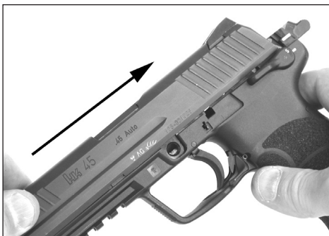
Figure 23 — Retract the slide
