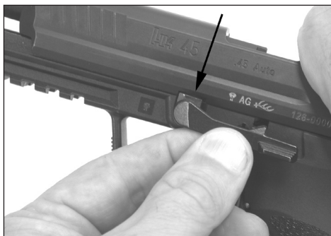
Figure 24 — Insert slide release
