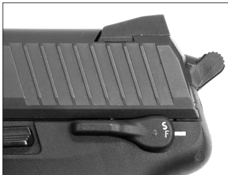
Figure 5 — Safety lever in "fire" position
