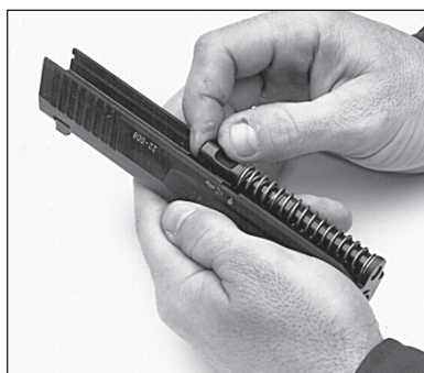
Fig. 18 – Recoil spring assembly in place
