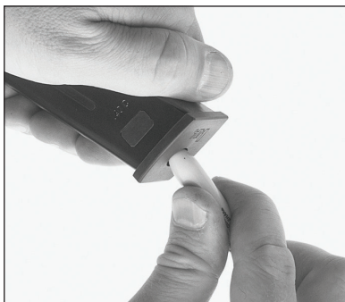
Fig. 21A – Depress locking detent 10-round magazine
