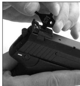
Fig. 28 Adjusting elevation screw
