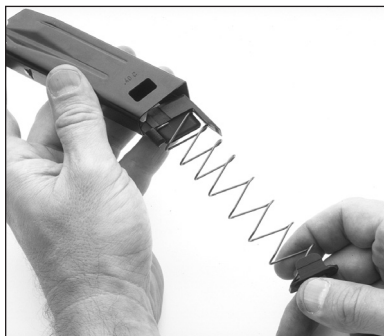
Fig. 21B – Removing floorplate 10-round magazine
