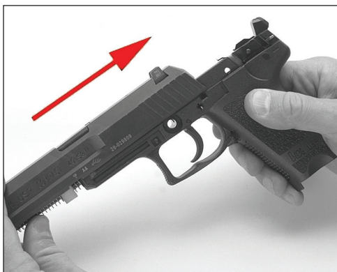
Fig. 20 – Slide back onto frame
