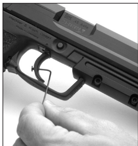
Fig. 26 Trigger stop adjustment with 1.5 mm Allen (hex) wrench
