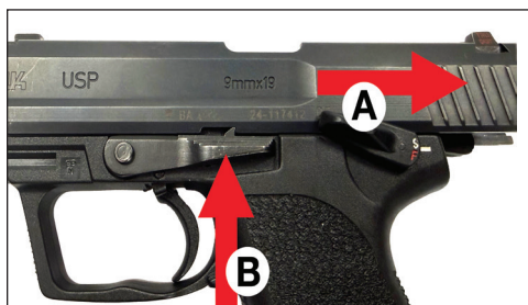
Fig. 11 – Locking the slide to the rear
