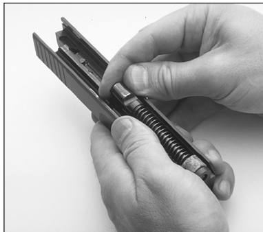
Fig. 15 – Separating barrel from slide
