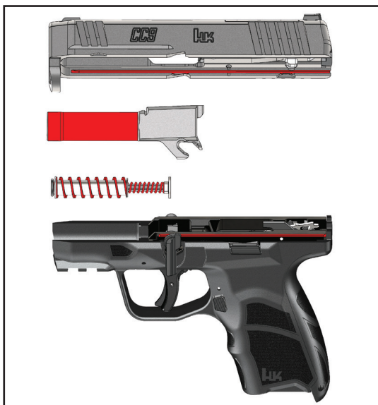
Figure 39 – Lubrication Points (in red)
