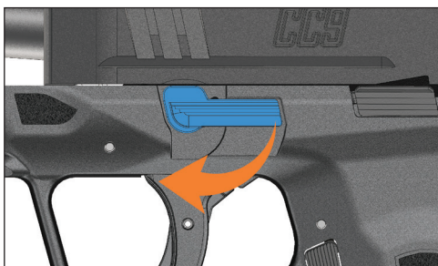
Figure 15 – Rotating the disassembly lever
