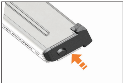
Figure 36 Hold the retainer flush with the magazine
