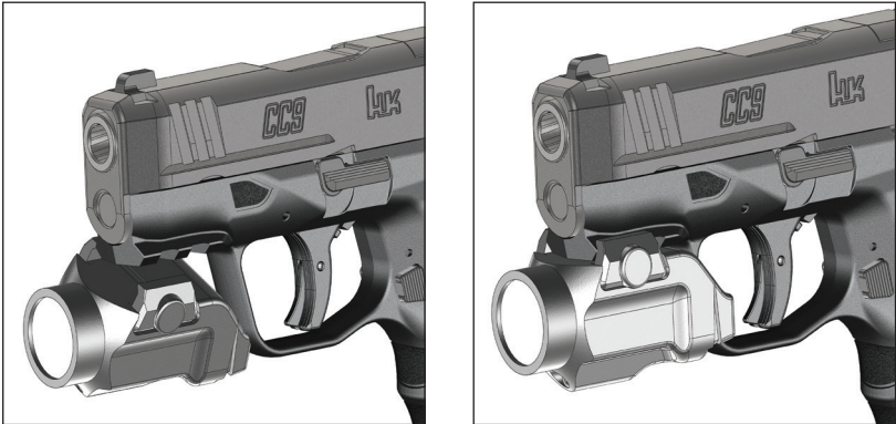
Figure 41 & 42 – Installing accessory lights onto the rails
