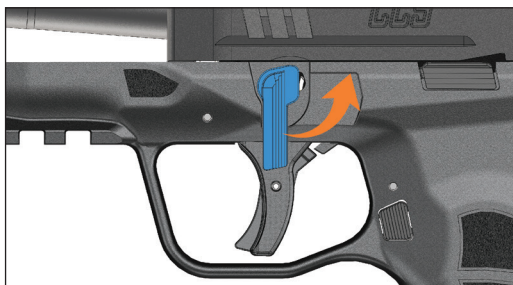
Figure 23 – Pivot the disassembly lever counterclockwise
