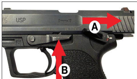
Fig. 11 – Locking the slide to the rear
