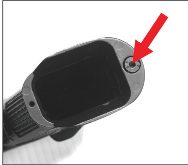
Fig. 32 HK Jet Funnel Allen wrench screw
