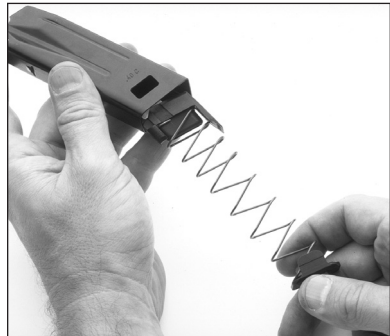
Fig. 21B – Removing floorplate 10-round magazine
