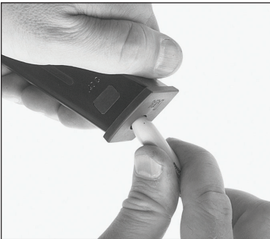
Fig. 21A – Depress locking detent 10-round magazine
