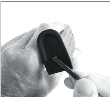
Fig. 22A – Depress locking detent 15-round magazine
