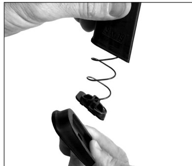
Fig. 22B – Removing floorplate 15-round magazine
