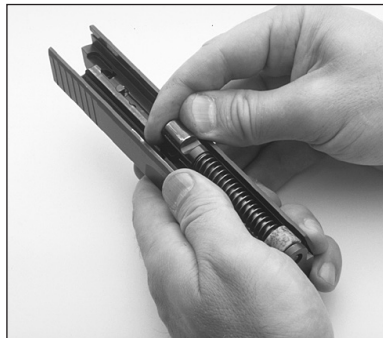
Fig. 15 – Separating barrel from slide
