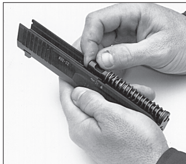
Fig. 18 – Recoil spring assembly in place
