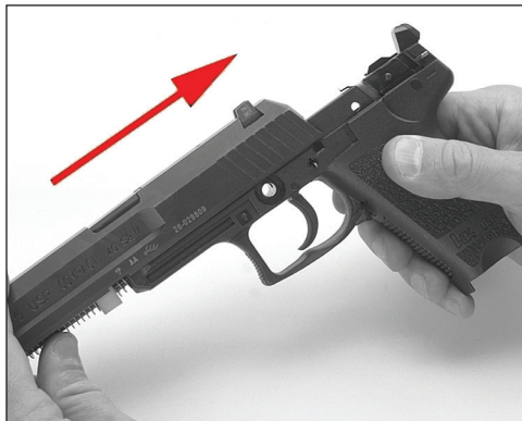
Fig. 20 – Slide back onto frame
