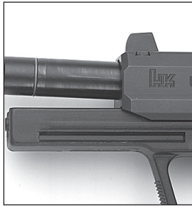
Fig. 30 O-ring shown on barrel
