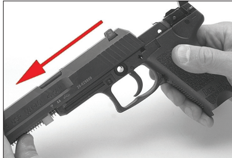
Fig. 14 – Remove the slide
