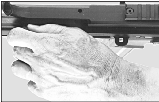
Fig. 20 Pull cocking lever backwards
