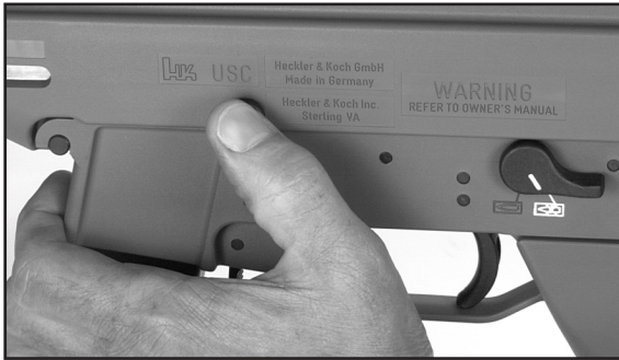
Fig. 21 Depress bolt catch to release the bolt
