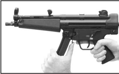
Fig. 23 – Depress the SP5 magazine release lever or button.
