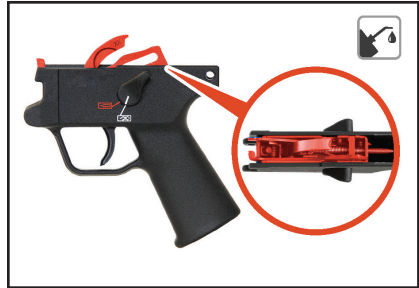
Fig. 55 – Lubrication points on pistol grip
