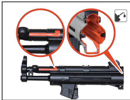
Fig. 56 – Lubrication points of functional elements
