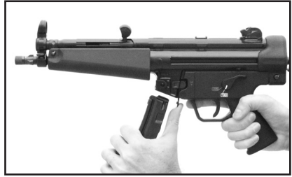
Fig. 34 – Remove the magazine from the magazine well.
