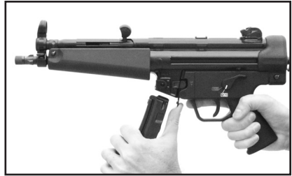
Fig. 24 – Remove the magazine from the magazine well.
