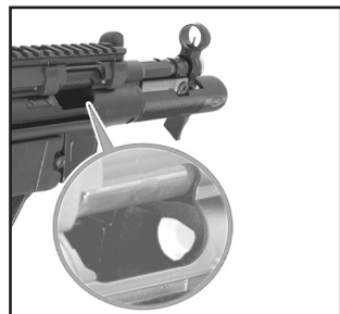
Fig. 22 – Check the chamber
