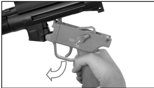
Fig. 36 – Remove pistol grip
