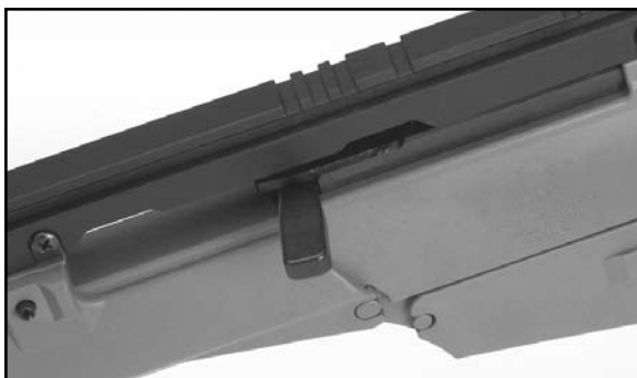
Figure 23 Cocking lever shown in its "forward assist" position
