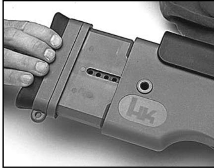
Figure 35 Remove buttplate with spacer
