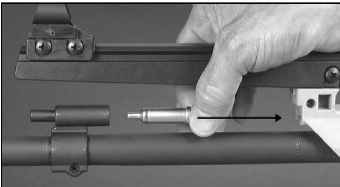
Figure 28 Removing the gas piston
