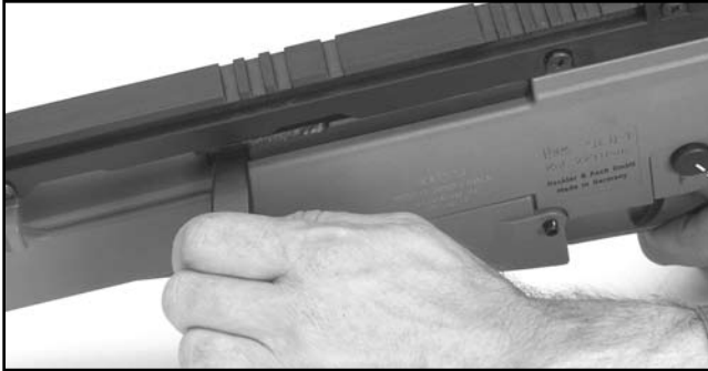
Figure 20 Operating the cocking lever
