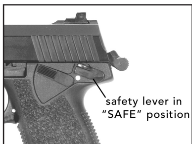
Figure 4 "Safe" Position (hammer cocked)
