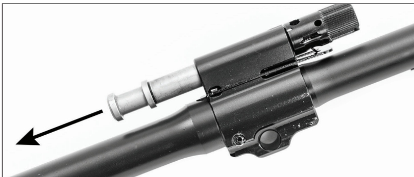
Fig. 26 – Removing Gas Piston
