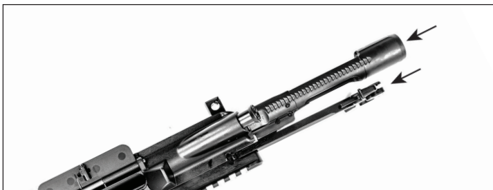
Fig. 38 – Installing the bolt carrier assembly into the upper receiver
