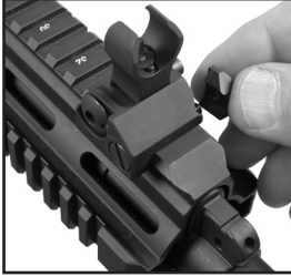
Fig. 6 – Installing front TROY sight
