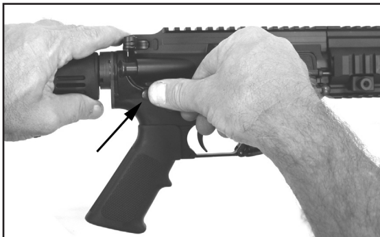
Fig. 99 – Completing the installation of the MR556A1 Upper Receiver on the Lower Receiver
