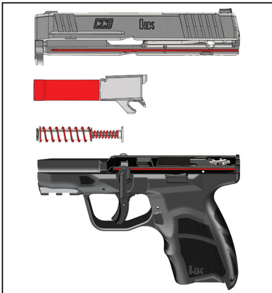
Figure 39 – Lubrication Points (in red)
