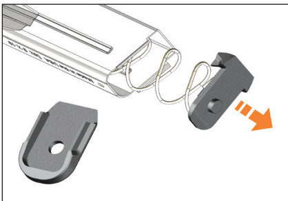
Figure 31 Removing locking plate and spring
