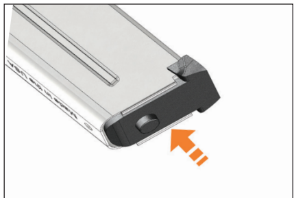
Figure 36 Hold the retainer flush with the magazine
