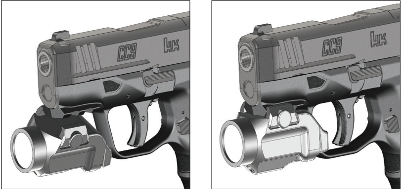
Figure 41 & 42 – Installing accessory lights onto the rails
