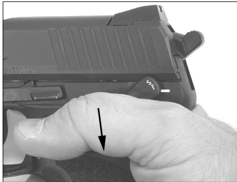
Figure 6 — Safety lever in "decocking" position
