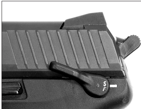
Figure 4 — Safety lever in "safe" position
