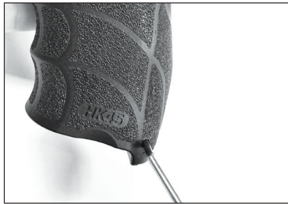
Figure 30 Tap the pin until fully seated
