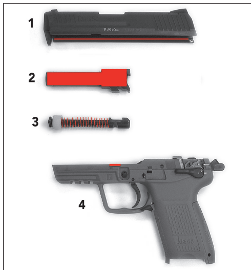
Figure 39 — Lubrication Points (in red)
