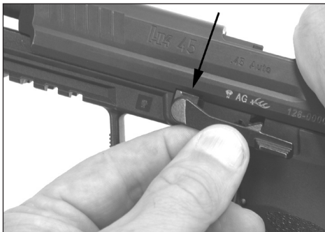
Figure 24 — Insert slide release
