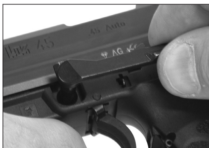
Figure 17 — Remove slide release
