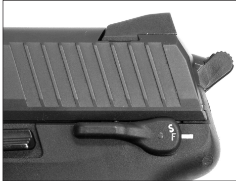
Figure 5 — Safety lever in "fire" position
