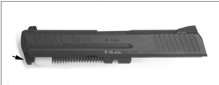
Figure 22 — Small hole in front of slide
