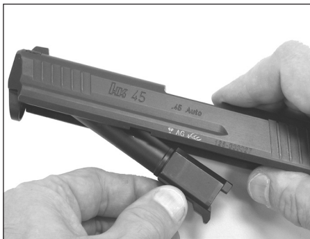
Figure 20 — Remove locking block
