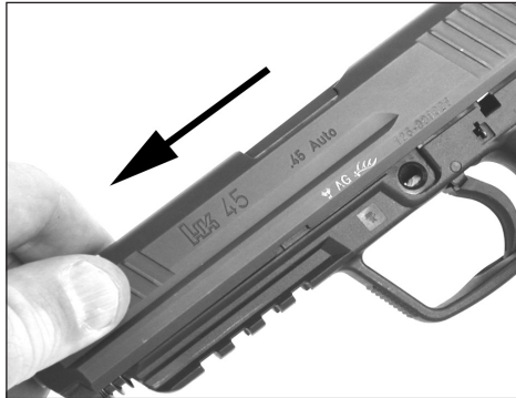
Figure 18 — Slide forward off frame
