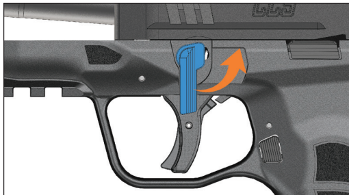
Figure 23 – Pivot the disassembly lever counterclockwise
