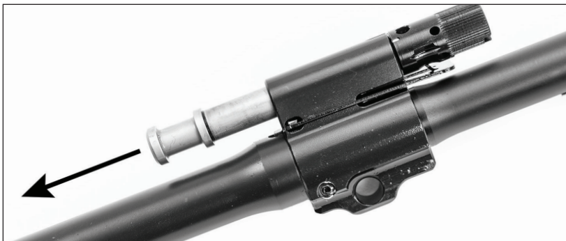
Fig. 26 – Removing Gas Piston
