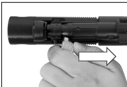
Fig. 20 – Move the bolt rearward
