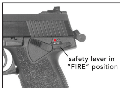
Figure 5 "Fire" Position (hammer cocked)
