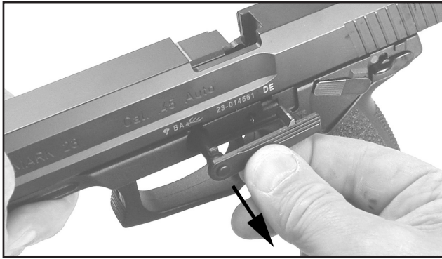
Figure 8 Removing the Slide Release
