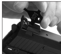
Fig. 30 Adjusting elevation screw
