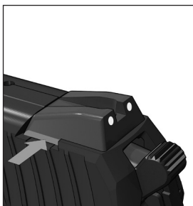
Fig. 7 Rear sight adjustment
