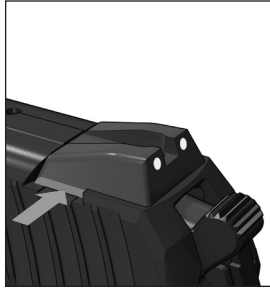
Fig. 7 Rear sight adjustment
