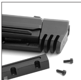
Fig. 36 Counterweight base and screws
