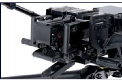
OPERATING ELEMENTS The safety/fire lever selector, trigger, and the charging handle are all located centrally on the end to the receivers
