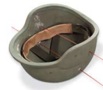
Kevlar helmet penetration at 200 meters. The same 4.6 mm cartridge easily passes through automobile windshields with minimal deflection.
