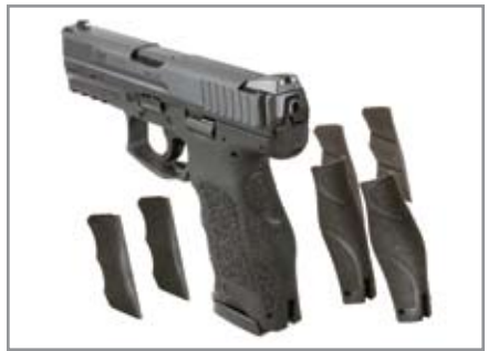
The VP9 uses striker fired ignition and a modified Browning operating system combined with an optimal "light pull" trigger control system — it is in essence a premium HK P30 frame mated to an advanced striker fired slide design. Advanced metallurgical and polymer materials include proprietary HK steel for barrel, slide, springs, pins, and other internal components. The VP9 polymer (polymer) frame is corrosion proof.
